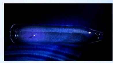
It generates a 253.7 nm emission line of an extremely narrow bandwidth which is congruent with the absorption line of the Hg atoms measured. The reference beam method is applied to get an exceedingly high stability of the UV source. The mercury concentration is measured in an optical cell which is made entirely of fused silica (Suprasil).
