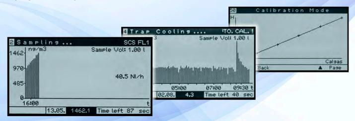
The results of the measurements are displayed on a graphic LCD as a graph and numerically. It is possible to view past readings with a paging function. Calibrations are stored in a non-volatile memory.
